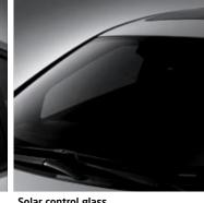
**Solar control glass**Reduces the penetration of heat rays for a cooler cabin.
